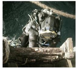
USS Bainbridge called to Souda bay with a damaged pit sword, the sub sea component of the pitometer log system. Aegean Diving Services rapidly mobilised to remove and replace with a new component. The whole operation took under 20 minutes from entering to exiting the water. This was yet another example of a combination of an experienced and professional diving team working in coordination with naval engineers to reach a common goal.
